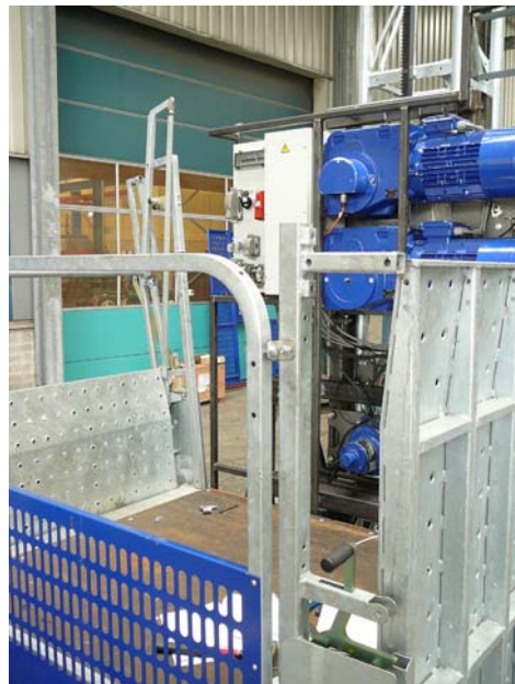
Connect all fences, bridge ramps etc.
