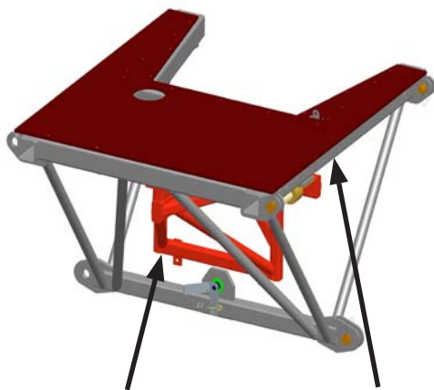
Support connected to Hinged deck
